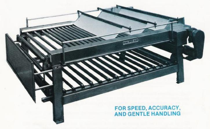
**SIMPLE DESIGN**—Easy to maintain, easy to adjust, with a unique patented method of roller expansion.
