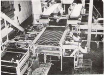
The versatile KERIAN SIZER adapts to almost any packing system. At the left is the KERIAN SIZER Model M-50 complete with cart, elevator, and reversible takeaway belts. At the right, the Model L-60 is installed after the grading tables and in front of a conveyor system which consists of six independently reversible belts.
